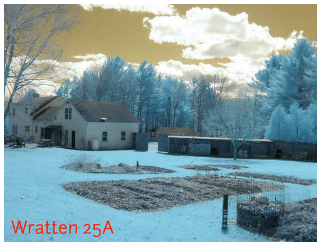
Replacing the infrared block filter with one that blocks blue and green but passes red and infrared allows photos that highlight plant health.
