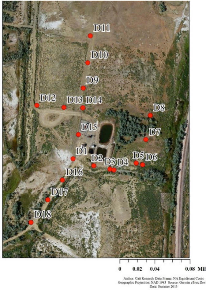
Figure 12: Photographic canisters testing locations on the Baker Ranch in Wyoming. Canisters were labeled and placed at set distances along roads surrounding a well. Image Courtesy of Caitlin Kennedy, 2013.
